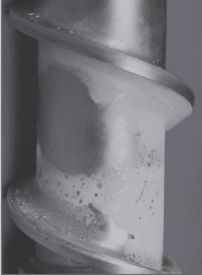
Extreme Scale Build Up on Evaporator Wall
