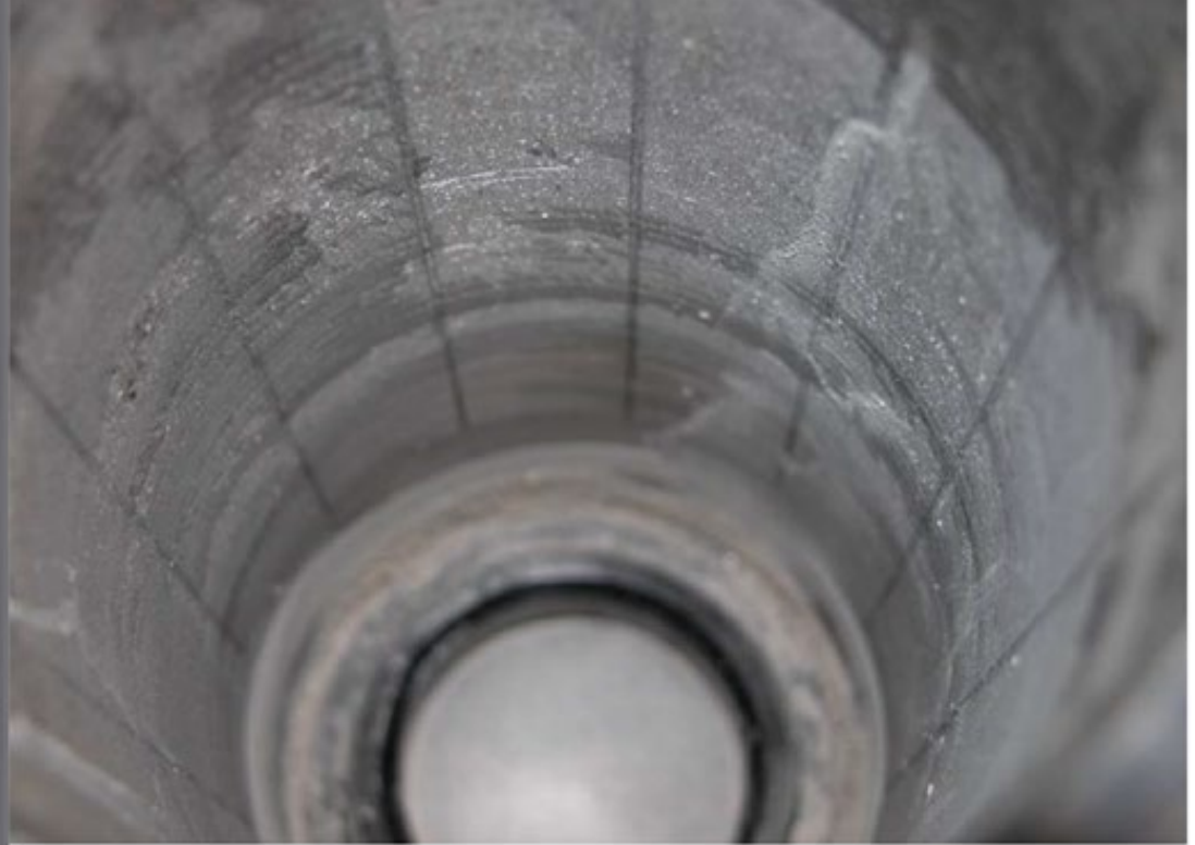
Extreme Scale Build Up on Evaporator Wall
